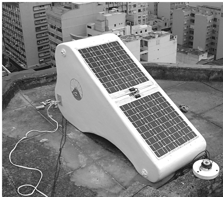
Figure 2. The All-in-One SHS during tests at Copacabana, Rio de Janeiro, Brazil.
