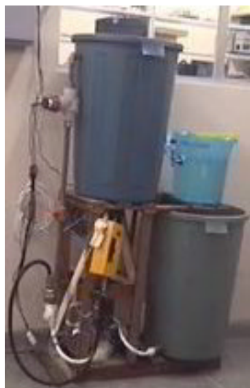
Fig. 3. PV-RO plant without batteries
